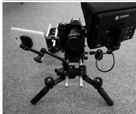
The portfolio of testing equipment includes remote controlled mounted stands, 15 m telescoping masts as well as shoulder mounted camera mounts. The measurements can be carried out to both panel and cell level, independent to the installation method or size, e.g. pitched-roofs, flat roofs, facades, and solar parks.
